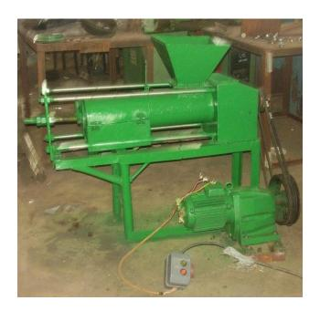
Figure 2: Palm oil screw press developed
